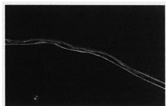
FIGURE 3. Light micrograph of nonhydrolyzed cotton stained with Congo red.
