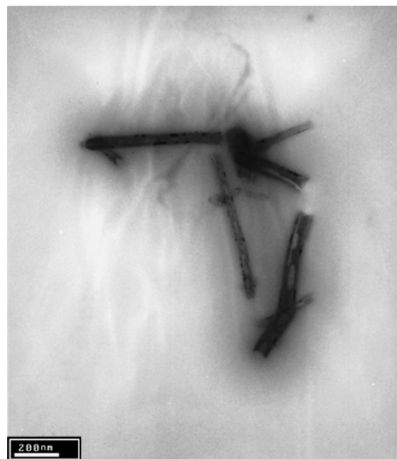
Figure 1 Transmission electronic microscope image of multi-walled carbon nanotubes.
