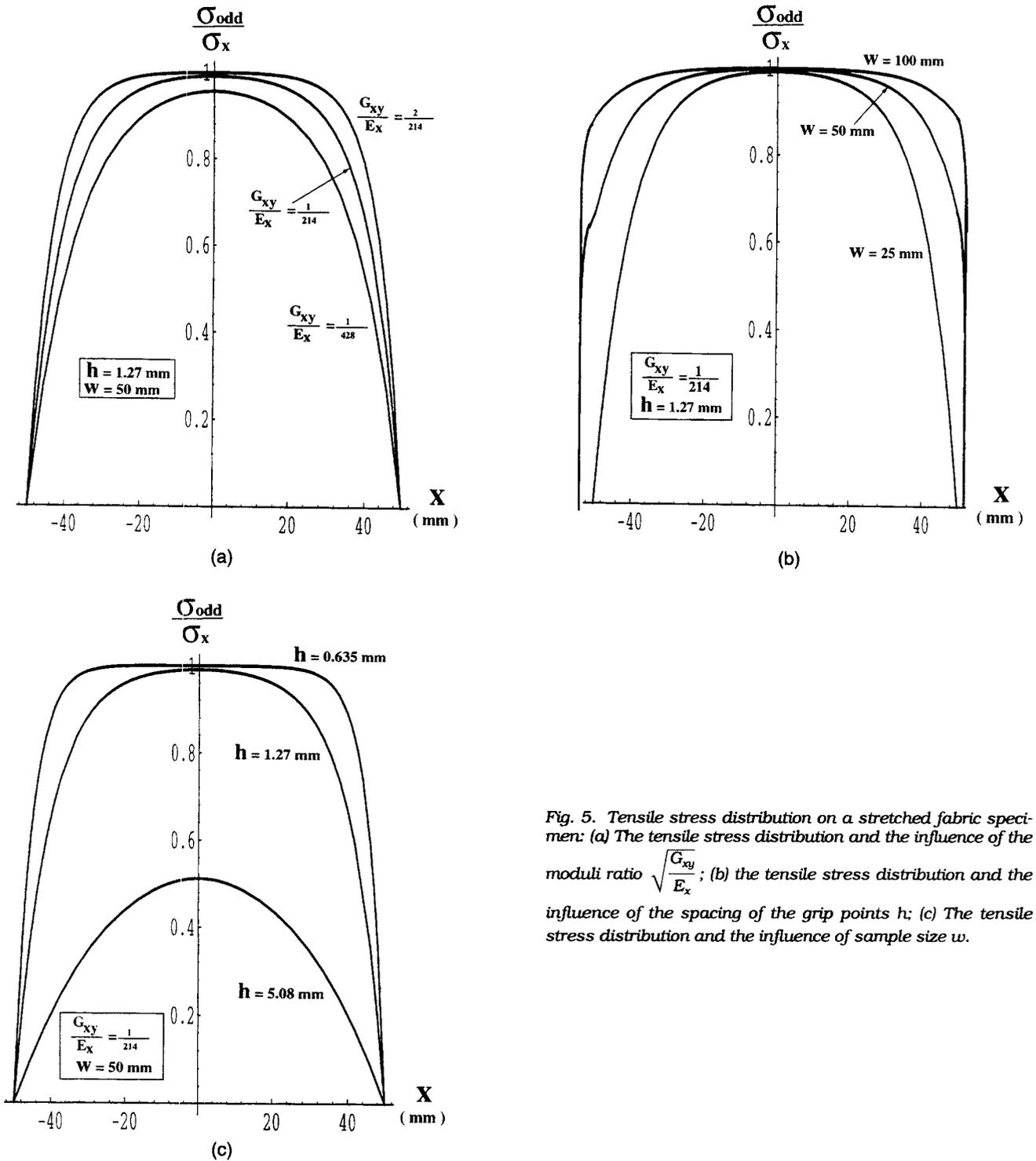
Fig. 5. Tensile stress distribution on a stretched fabric specimen: (a) The tensile stress distribution and the influence of the moduli ratio  $\sqrt{\frac{G_{xy}}{E_x}}$ ; (b) the tensile stress distribution and the influence of the spacing of the grip points  $h$ ; (c) The tensile stress distribution and the influence of sample size  $w$ .
