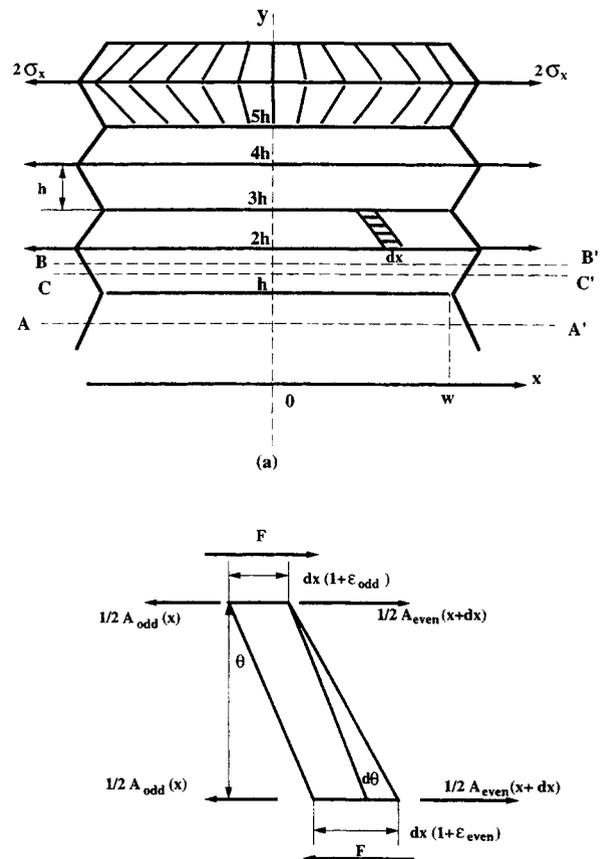
Fig. 2. A stretched fabric specimen: (a) A fabric specimen gripped at discrete points along opposite edges; (b) A yarn segment from the stretched specimen.
