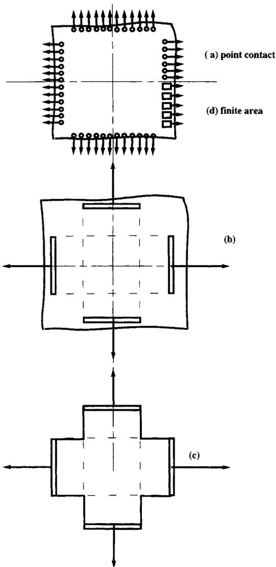
Fig. 1. Different types of biaxial fabric testers: (a) Point gripping; (b) Grab test; (c) Cruciform test; (d) Segmented clamps.
