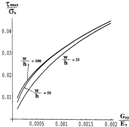
Fig. 4. The relative maximum shear stress  $\frac{\tau_{max}}{\sigma_x}$  and the related parameters.
