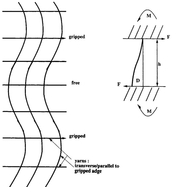
value, for the fabric in *Table 1* where sample length  $2w = 100$ , this value  $h = 1.3$  mm (or 20 grip points per inch). Grip point spacing is less critical when woven specimens are mounted at bias angles.
