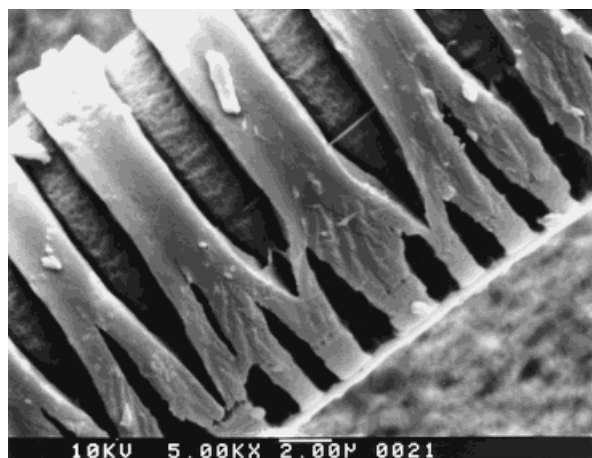
Figure 4 Scanning electron micrograph of hydrolyzed BD; weight loss = 14.6%.
