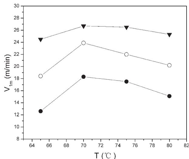
**Figure 6** Relations between  $V_{1m}$  and spinning temperature  $T$ . The water content in spinning solution: ▼—0 wt %, ○—2 wt %, and ●—4 wt %. The concentration of spinning solution was 20 wt %. The coagulating bath concentration and temperature were 50 wt % and 20°C, respectively. The air gap length was 30 mm.
