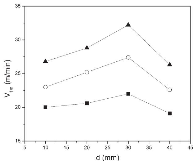
**Figure 4** Relations between  $V_{1m}$  and the air gap length  $d$ . The concentration of spinning solution: ■—17 wt %, ○—20 wt %, and ▲—23 wt %. The coagulating bath concentration and temperature were 50 wt % and 20°C, respectively. The spinning temperature was 70°C.
