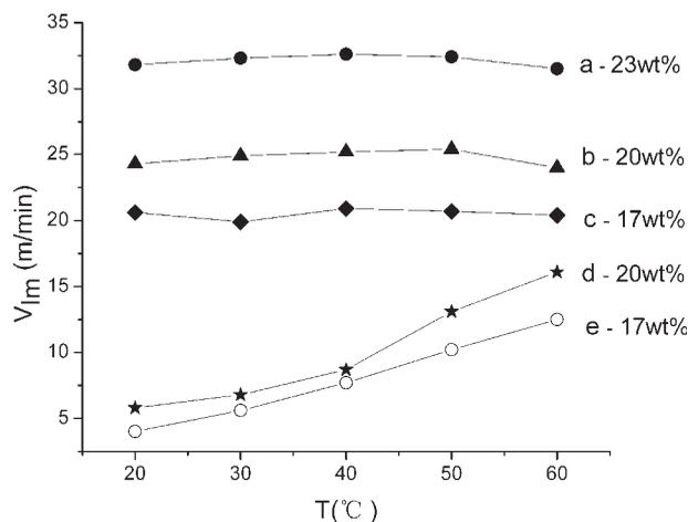
**Figure 2** Relations between the coagulating bath temperature  $T$  and  $V_{1m}$ . The spinning temperature was  $70^\circ\text{C}$  and the coagulating bath concentration was 50 wt %, air gap length 30 mm (for dry-jet wet spinning).
