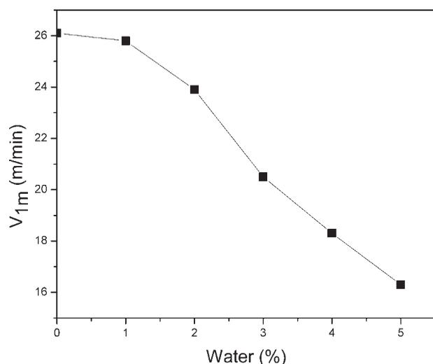
**Figure 5** Relation between  $V_{1m}$  and the water content in spinning solution. The coagulating bath concentration and temperature were 50 wt % and 20°C, respectively. The concentration of spinning solution was 20 wt %, and the spinning temperature was 70°C. The air gap length was 30 mm.
