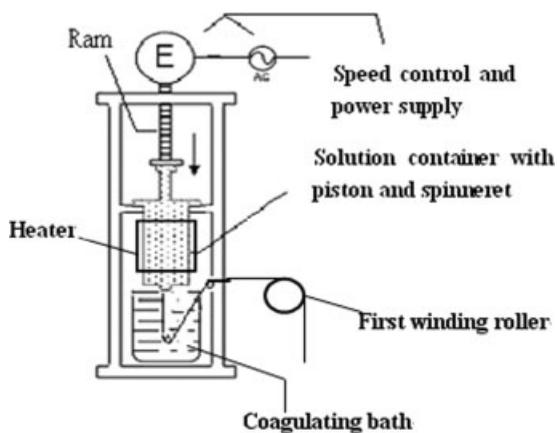
**Figure 1** Sketch of the experimental spinning machine.
