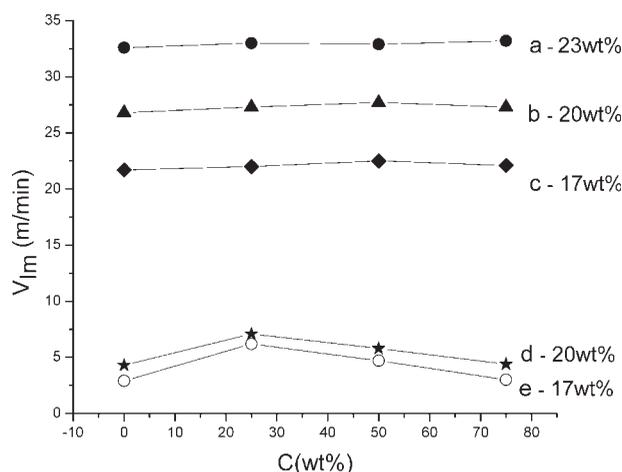
**Figure 3** Relations between the coagulating bath concentration  $C$  and  $V_{1m}$ . The spinning temperature was  $70^\circ\text{C}$ , the coagulating bath temperature  $20^\circ\text{C}$ , air gap length 30 mm (for dry-jet wet spinning).
