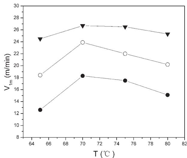
**Figure 6** Relations between  $V_{1m}$  and spinning temperature  $T$ . The water content in spinning solution: ▼—0 wt %, ○—2 wt %, and ●—4 wt %. The concentration of spinning solution was 20 wt %. The coagulating bath concentration and temperature were 50 wt % and 20°C, respectively. The air gap length was 30 mm.
