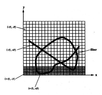
Fig. 2 The co-ordinate system, the lattice and various spin cells
