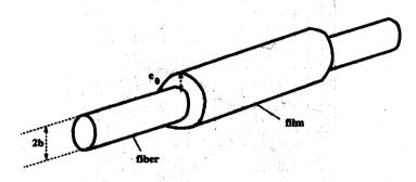
Fig. 1 A fiber of radius b covered by liquid film of equilibrium thickness e,
