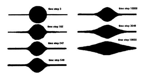
Fig. 7 Simulation of the spreading of a liquid drop on a fiber
