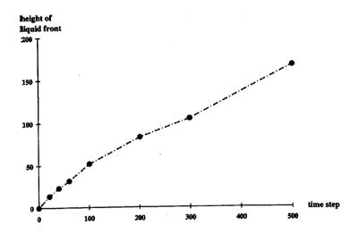
Fig. 5 The wetting simulation results in relative units: (a) Wetting progress with time in a fiber network; (b) Change of the height of the liquid front during wetting
